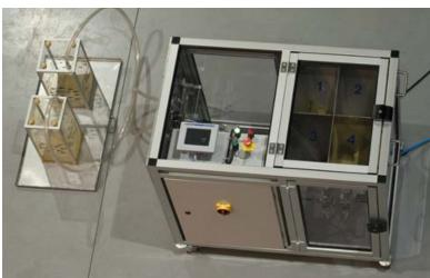
Automatic central feeding System of microdiets for juvenile and larval fishes Microdiets from 75 μm | Up to 60 tanks | Doses from 5 grams
